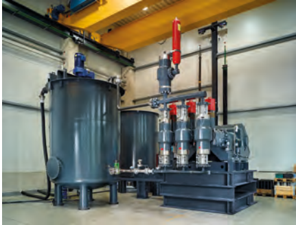
Figure 1: FELUWA slurry test rig Performance data: Q=14 m 3 /h, p=130 bar(g)
